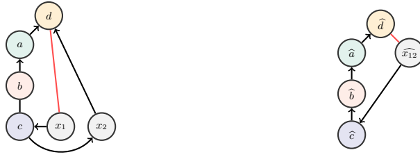
Fig. 3: Concrete network (left) and its corresponding \forall\exists -abstraction (right). Node c prefers to route through x_1, x_2 and nodes x_1, x_2 prefer to route through c .
